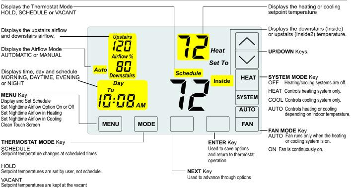
Setpoint temperatures are kept at the v temperatures set by the installer.
