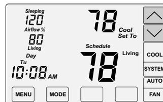
Touch the UP/DOWN keys to adjust the setpoint temperature.
